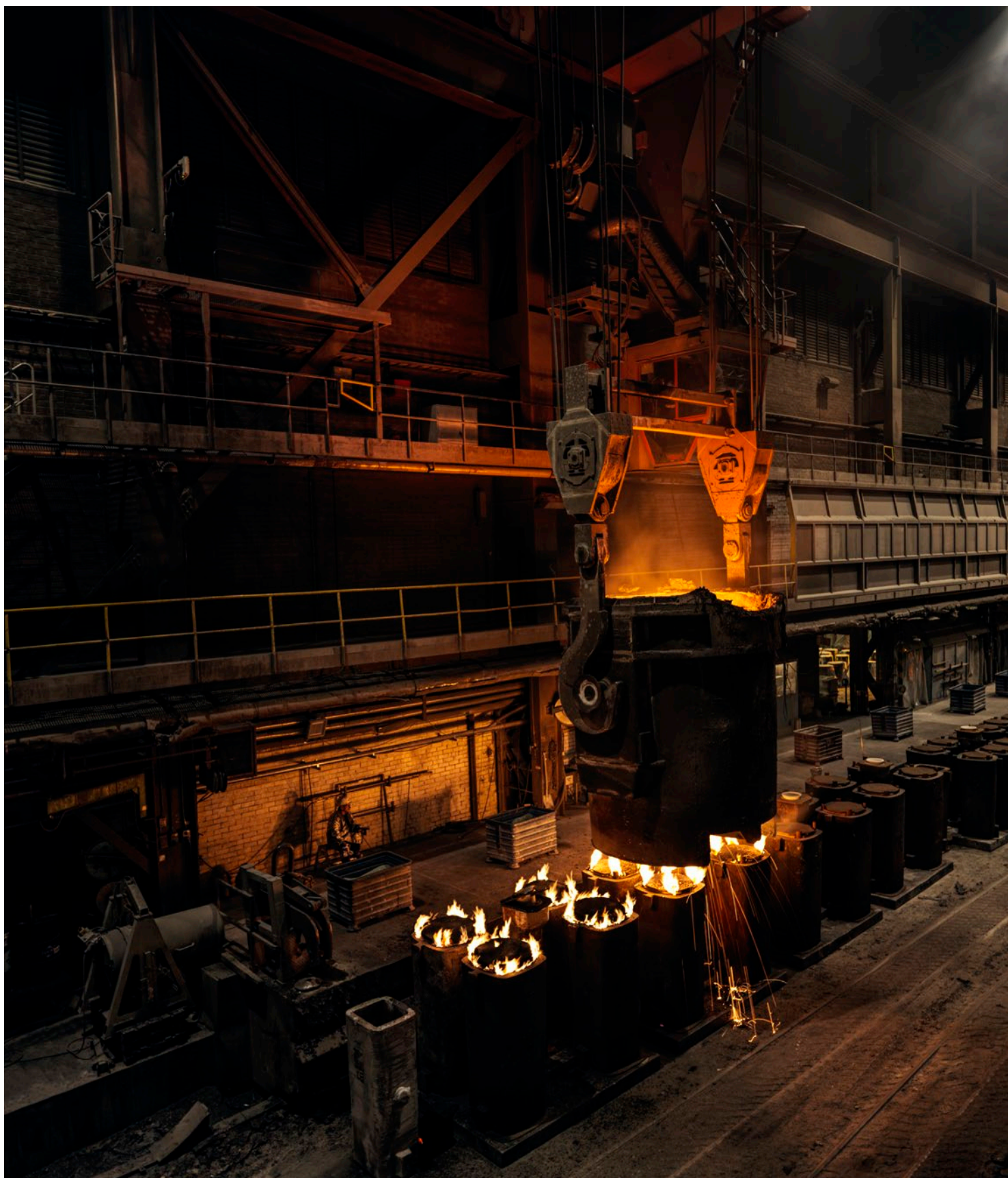
Bloom casting at the steel mill in Sandviken, Sweden. Special alloys for advanced applications within the energy sector, such as nickel base and duplex steels, are among the materials produced here.
