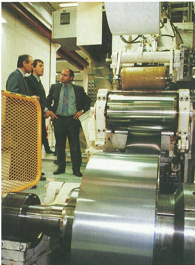
During 1994, a new cold-rolling mill was placed in service in Sandviken. The new facility will increase production of very thin strip, used primarily for razor blades and in catalytic converters for cars. The inauguration of the new mill was attended by representatives of some of Sandvik's major customers.
