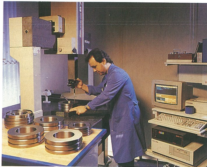
When Sandvik's cemented-carbide rolls undergo final inspection, the inspection record includes measurement data for each roll.
