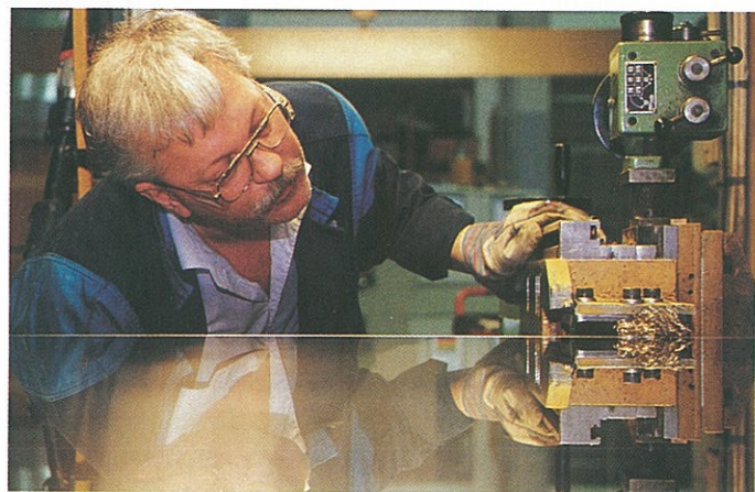
Edge treatment is an important process in the manufacture of wide steel belts at Sandviken. Bengt Forsberg checks the quality of the end product.
