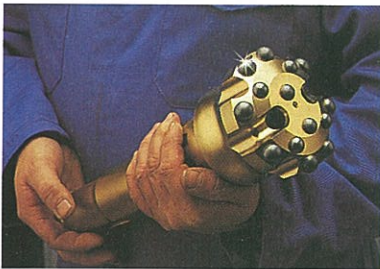
Diamond-coated cemented-carbide buttons have dramatically improved the wear-resistance of drill bits of this type.
