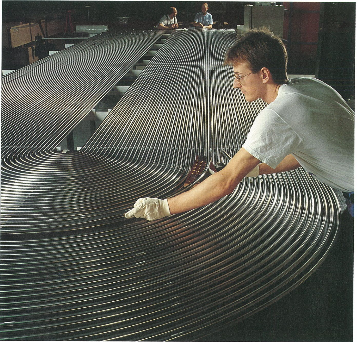
Steam -generator tubes for nuclear power stations are a typical example of high added-value steel products for a special product niche, in which Sandvik Steel is a leader.
