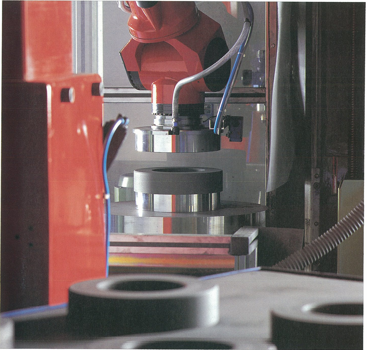
Robots are used in the manufacture of blanks produced in the automated cemented-carbide hot-rolls production line of Sandvik Hard Materials to improve product quality and the work environment.
